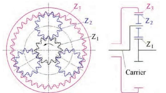
Figure 1: Epicyclic stage with singular planet gears; numbers of teeth:  $z_1$  — sun gear,  $z_2$  — planet gear, and  $z_3$  — ring gear
