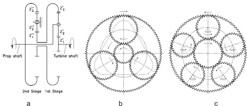
Figure 8: (a) TV7-117S gearbox arrangement; (b) first and (c) second stage sections
