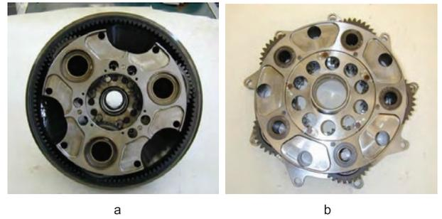
Figure 9: Assemblies of (a) first and (b) second stages of TV7-117S turboprop engine gearbox
