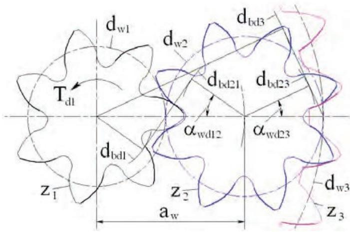
Figure 3: Epicyclic mesh with singular planet gears
