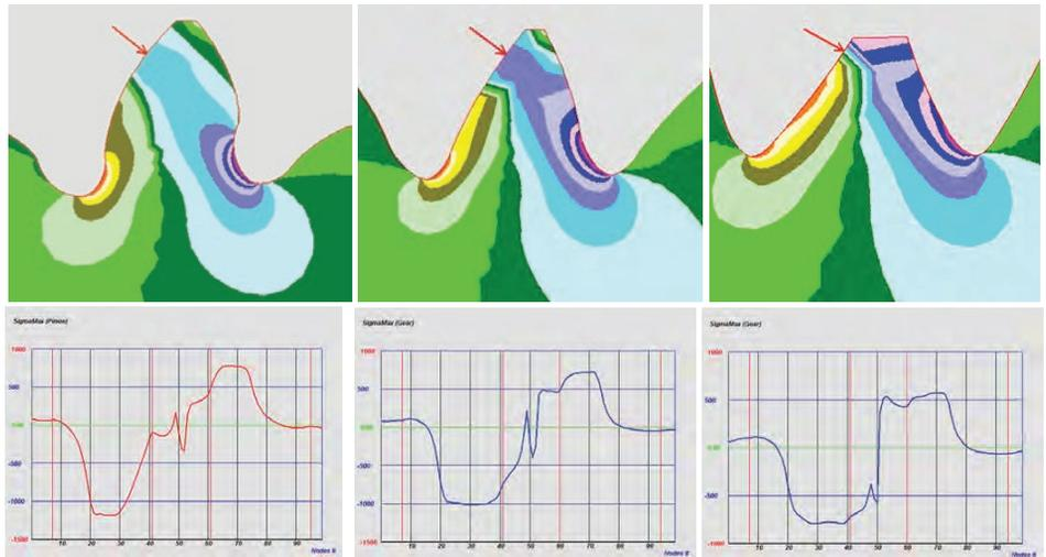
Figure 7: (a) Asymmetric epicyclic gear stage stress isograms; (b) charts of sun gear, planet gear, and ring gear respectively
