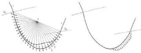
Figure 5: Tooth root fillet optimization: a — profile shaping technique, b — stress chart; 1 — involute tooth flanks, 2 — initial fillet profile, 3 — fillet center, 4 — optimized fillet profile,  $d_{fd}$ ,  $d_{fc}$  — form circle diameters of the drive and coast tooth flanks
