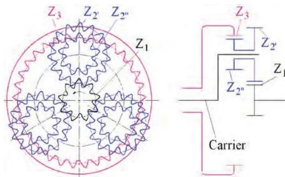
Figure 2: Epicyclic stage with compound planet gears; numbers of teeth:  $z_1$  — sun gear,  $z_2$  — planet gear portion engaged with sun gear,  $z_2''$  — planet gear portion engaged with ring gear, and  $z_3$  — ring gear
