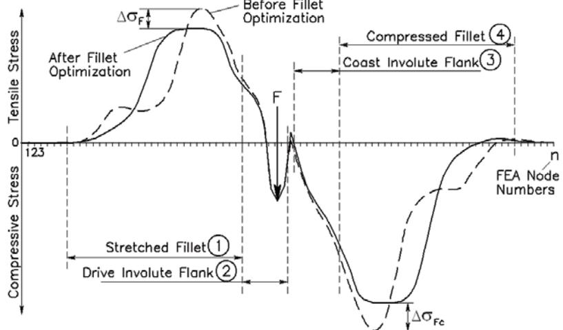
Figure 6: Tooth stress distribution comparison before and after root fillet optimization: a — tooth FEA mesh, b — stress distribution charts,  $\Delta\sigma_F$  — tensile stress reduction,  $\Delta\sigma_{Fc}$  — compressive stress reduction
